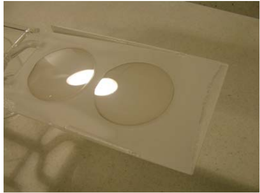
Fig.1: Large area wafer capability. View of two 120 \mu\text{m} thick GaN wafers fabricated on 100-mm c-plane sapphire.
