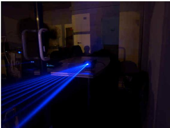
19 keV. The duration of the light pulse was  $\sim 100 \text{ ns}$ , the wavelength at the maximum of the line - 438 nm. The maximum peak power of about 2 W was obtained at an electron energy of 25 keV.
